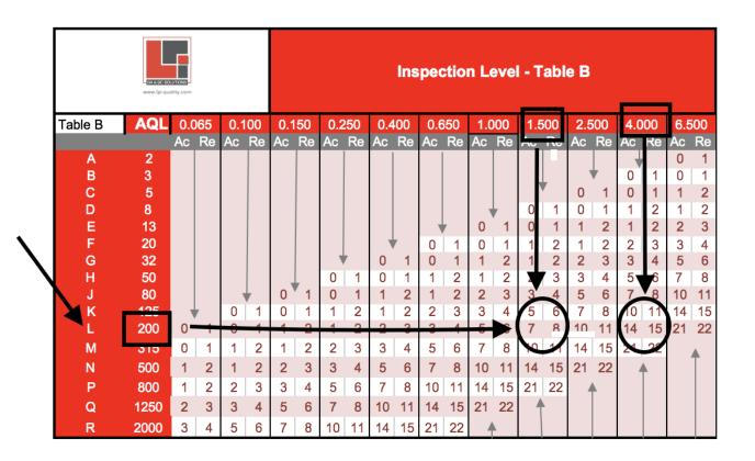
This table is used to find the specific sampling plan, including the number of samples to be inspected and the acceptance/rejection criteria based on the AQL.
